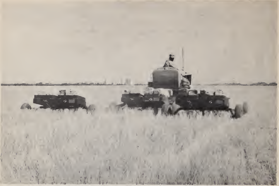
FIGURE 1.—Undercutting wheat stubble in preparation for next year's grain sorghum. Volunteer wheat and weeds are killed and plant cover prevents soil blowing. Rainfall and snow conservation will be high.
